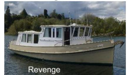
She is of carvel plank counter stern design, built of kauri with puriri cross floors and pohutakawa ribs and is fixed by copper nails and roves.
